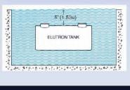
tube is welded liquid tight into steel tank. In the event of a breach to the inner or outer wall, the intruding liquid flows into the monitor access tube. Any liquid in contact with the electronic sensor probe will trigger alarm.
